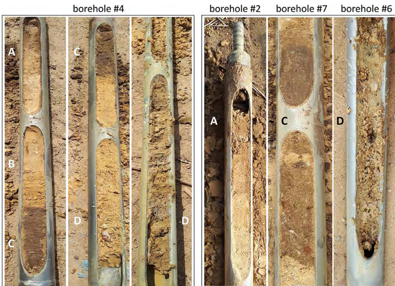
Fig. 5 Photographs of boreholes with an indication of the identified sedimentary units. Each metal window represents a 50 cm long interval of sediments (photos W. Toonen, J. Krejčí)
